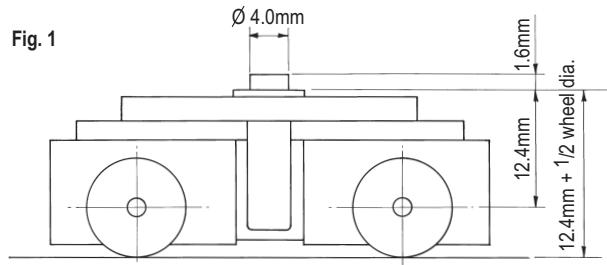
If the height does not suit, it may be necessary to cut an opening in the floor which is then filled with an adaptor plate made from 1.5mm or 0.060" polystyrene or brass sheet.
